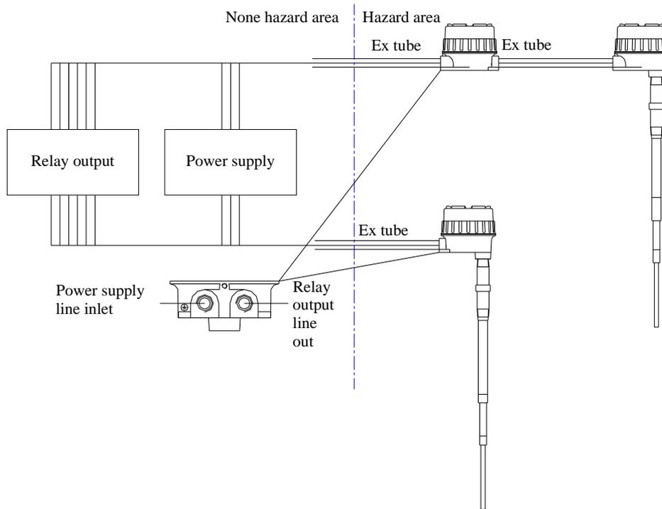
Figure 4.4 System wiring
