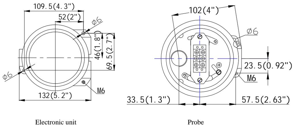
Figure 4.3 XP housing installation
