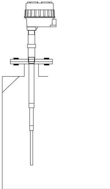
**Bracket mounting in open vessel**
