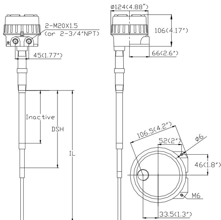
Figure 4.1 AVI-PDU integral system mounting
