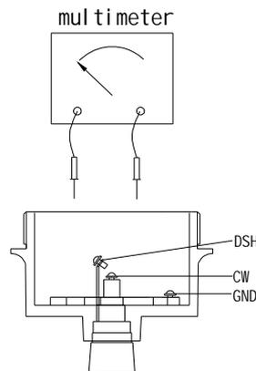
7.2 Testing sensing element
