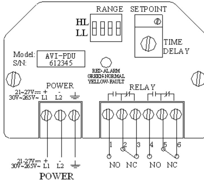
Figure 4.9 power wiring
